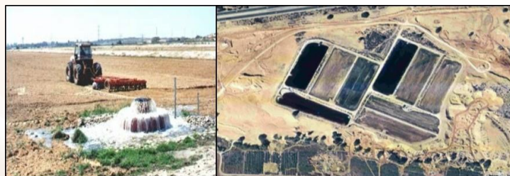
Figure 2 – SAT : Soil Aquifer Treatment
